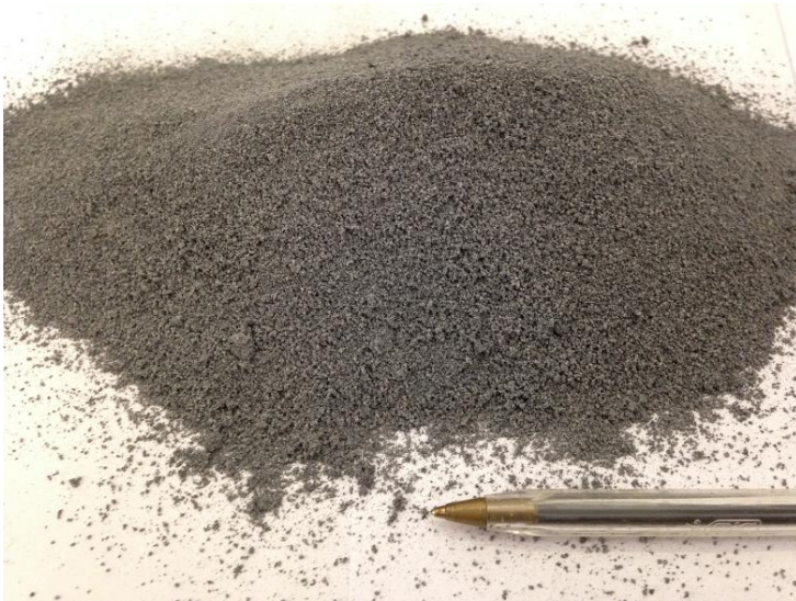
Figure 3: Components – Aspect of Reacted and Activated Rubber
