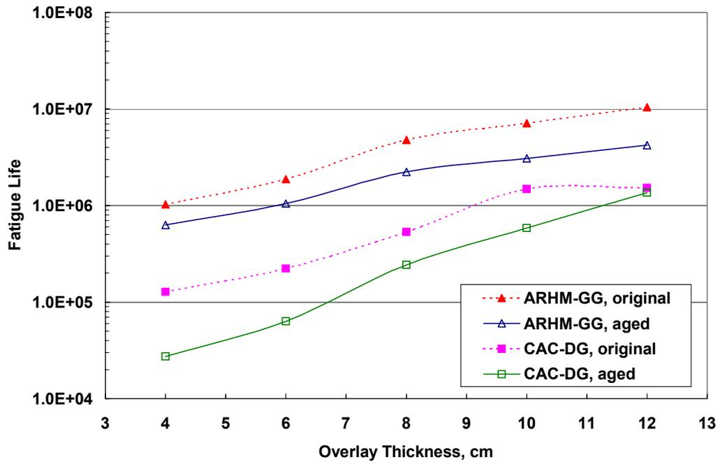
FIGURE 10 Fatigue life variation for overlay construction (distortion energy criterion).
