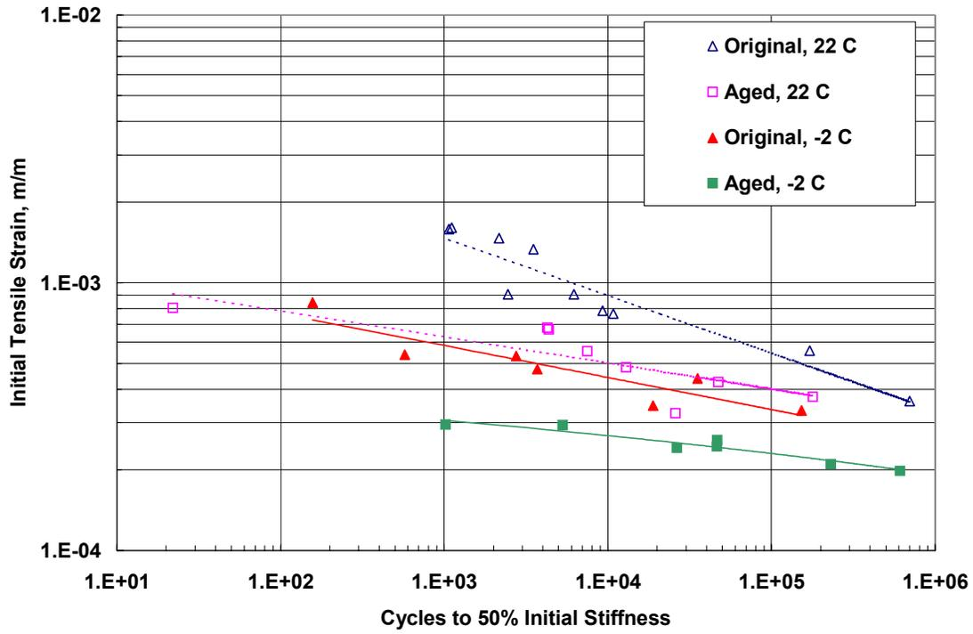
FIGURE 2 Fatigue relationships for CAC-DG using tensile strain criterion.
