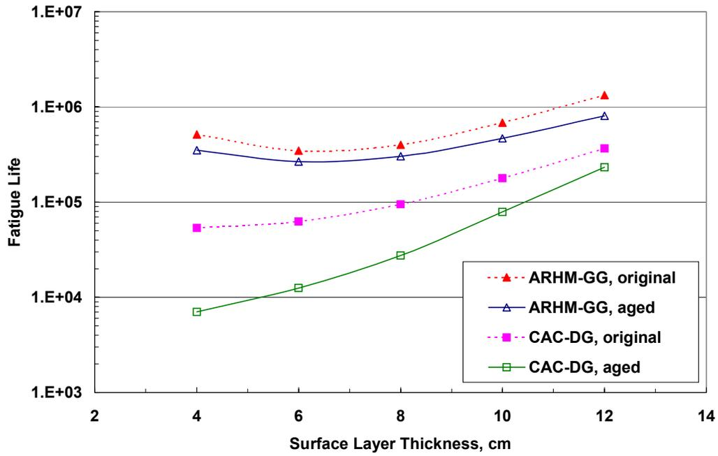
FIGURE 8 Fatigue life variation for new pavement construction (distortion energy criterion).
