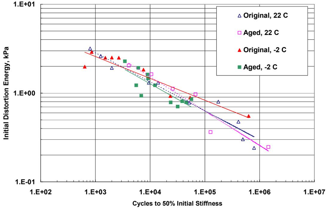
FIGURE 5 Fatigue relationships for ARHM-GG using distortion energy criterion.
