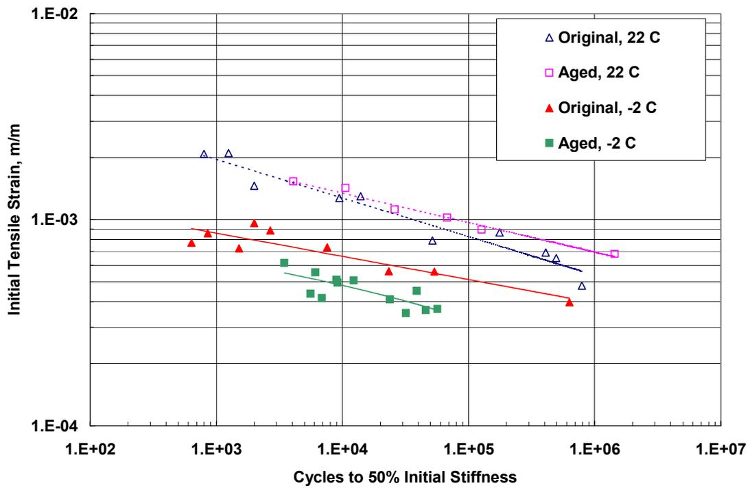
FIGURE 3 Fatigue relationships for ARHM-GG using tensile strain criterion.
