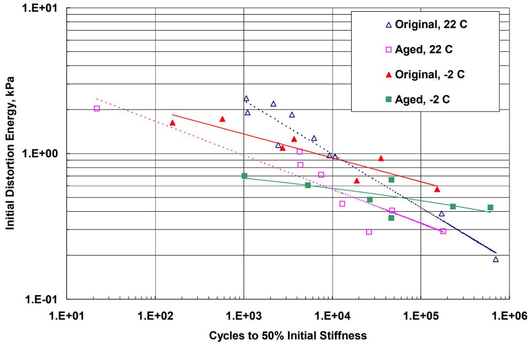
FIGURE 4 Fatigue relationships for CAC-DG using distortion energy criterion.
