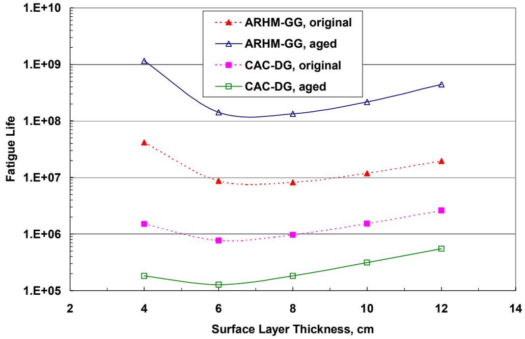
FIGURE 7 Fatigue life variation for new pavement construction (tensile strain criterion).
