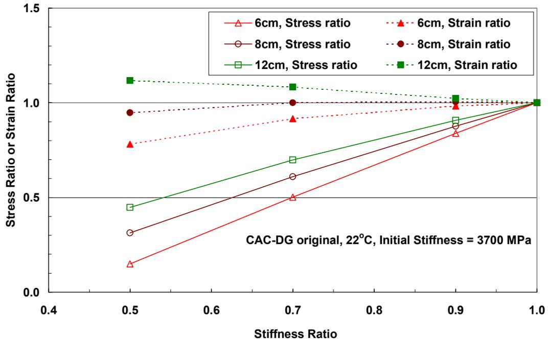
FIGURE 6 Stress or strain ratio variation with stiffness ratio for different overlay thicknesses.
