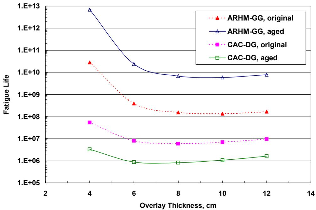
FIGURE 9 Fatigue life variation for overlay construction (tensile strain criterion).
